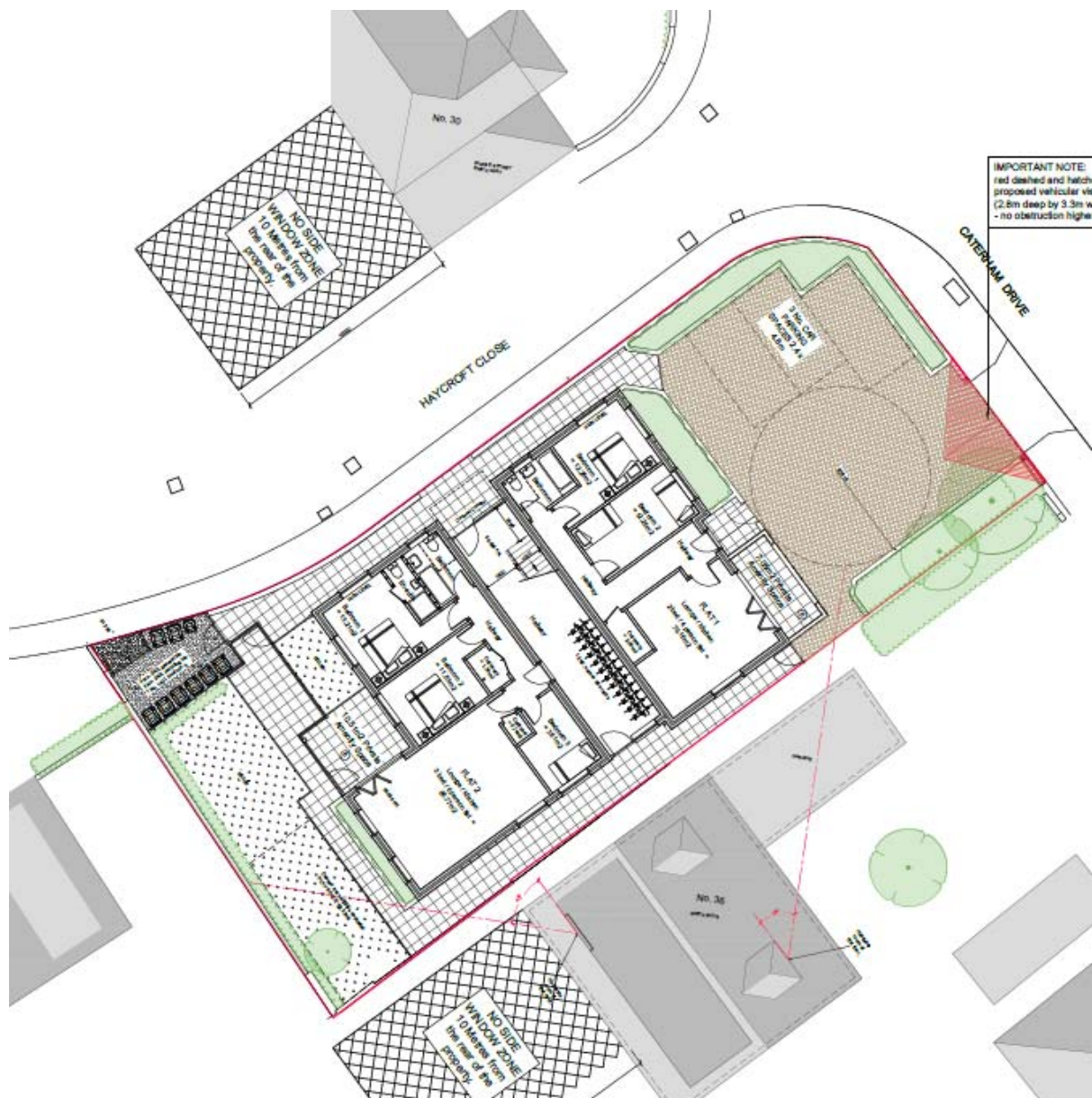
Fig 5: Ground floor plan proposed site showing proposal in relation to neighbouring properties
