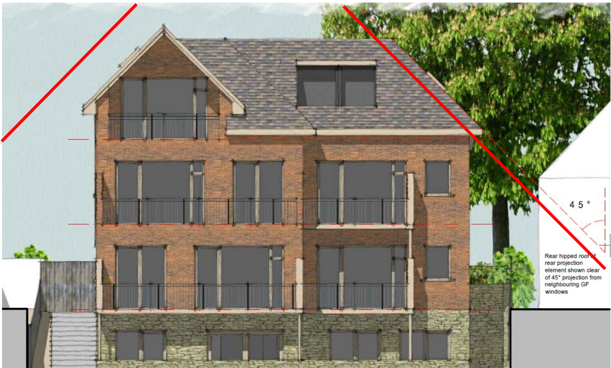
Figure 8: Rear elevation with 45 degree line
